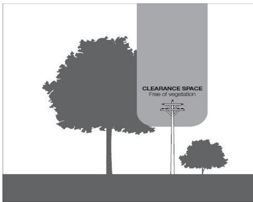
Figure 5—Uninsulated 66 000 volt electric line in a low bushfire risk area and uninsulated electric line in a hazardous bushfire risk area
