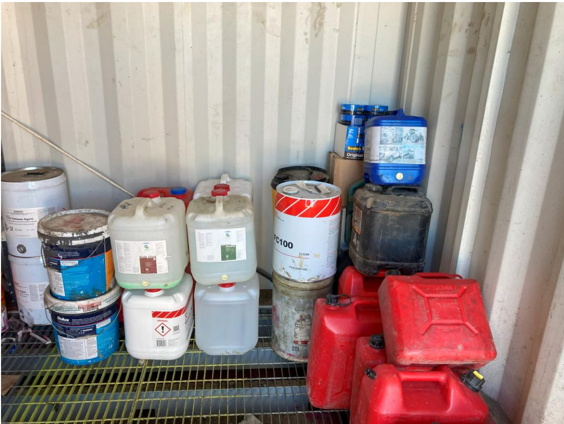
Plate 4 – Bunded container used for chemical storage at Stage 2
