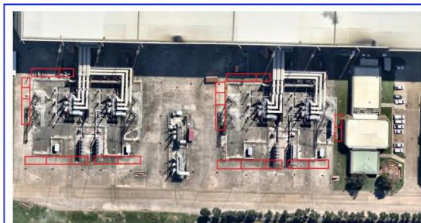
Figure 4 Indicative configuration of the temporary shipping container to form a blast wall
