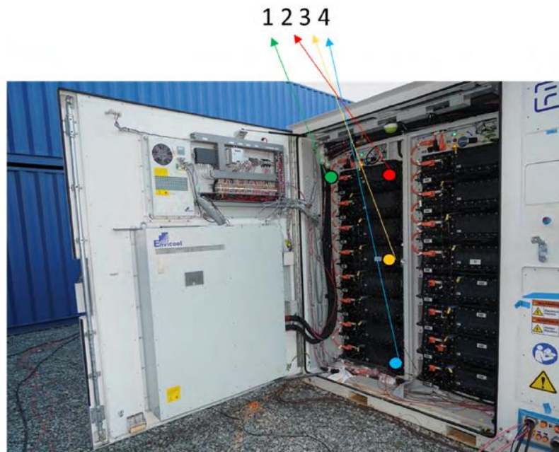
Figure 2-13: Target Unit 3: thermocouple positions
