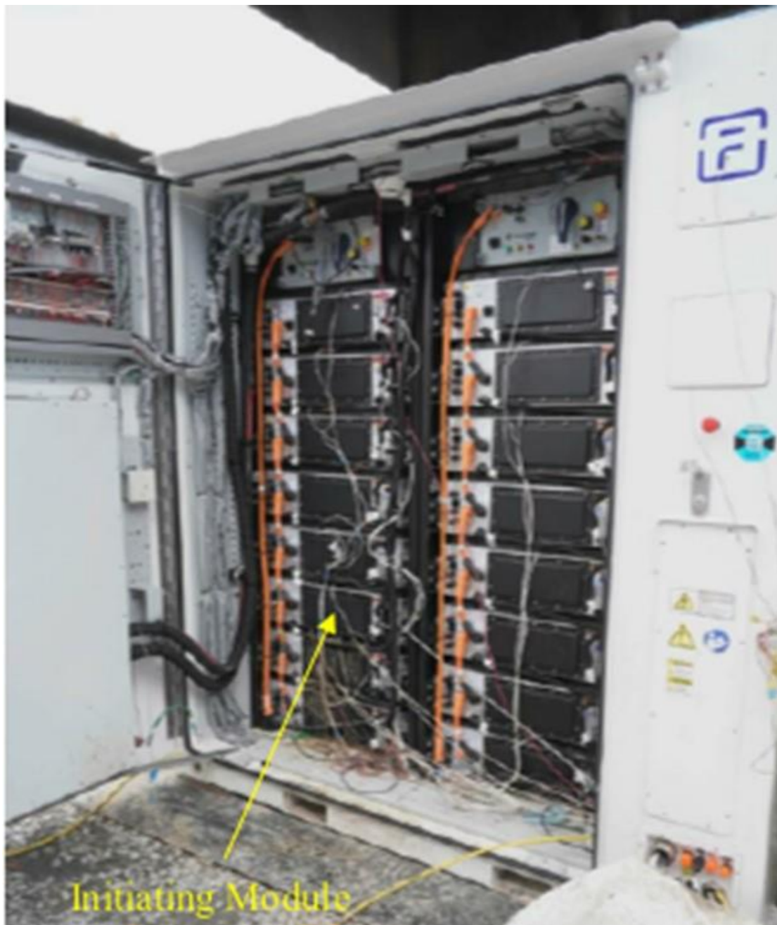
Plate 6: Initiating Unit: interior after the test
