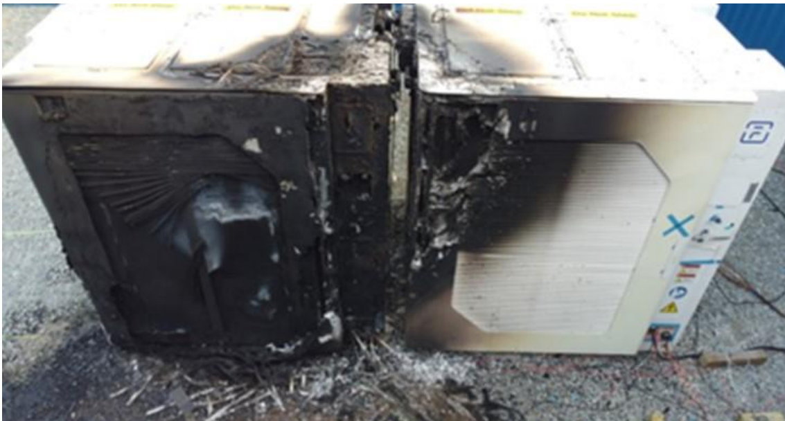
Figure 2-26: Damage sustained to Cubes in the Bespoke Burn test
