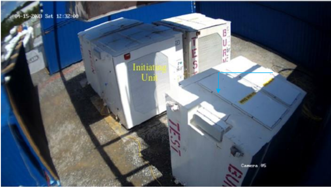
Plate 3: Unit level test set-up: UL 9540A test (Ref 15)
