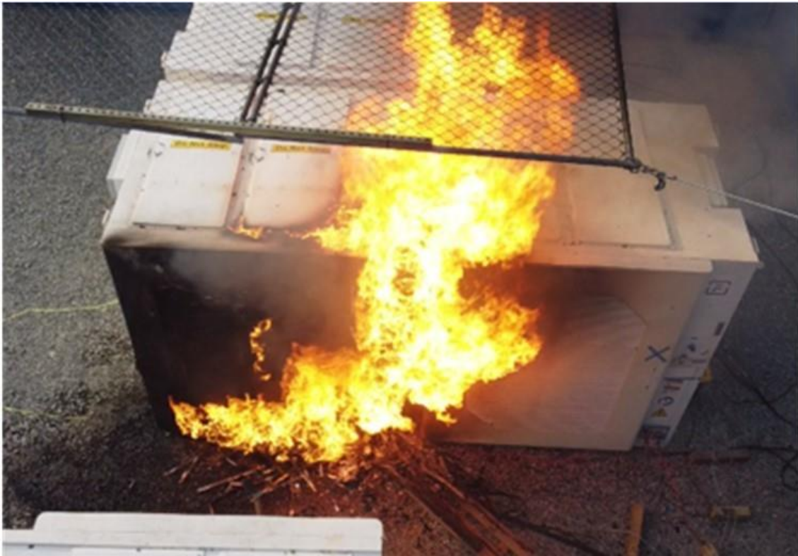
Figure 2-25: Flames tilting across the directly adjacent Cube due to wind in the Bespoke Burn test
