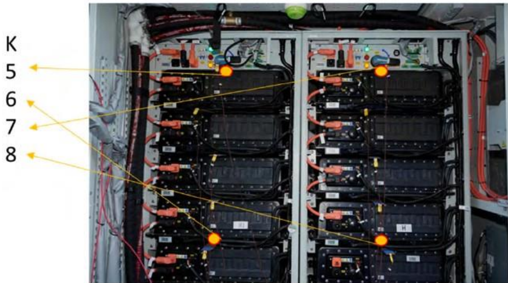
Figure 2-11: Target Unit 1: thermocouple positions
