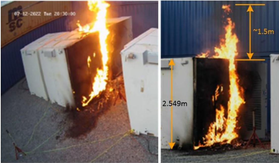
Figure 4-1: Flames extending above the roof line of the Cube in the Bespoke Burn test
