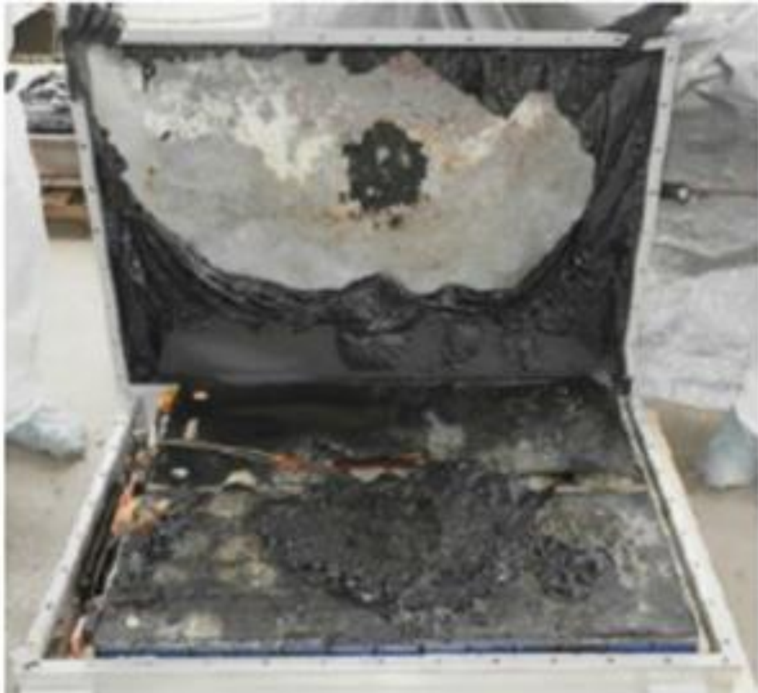
Plate 5: Initiating module: after the test, lid removed
