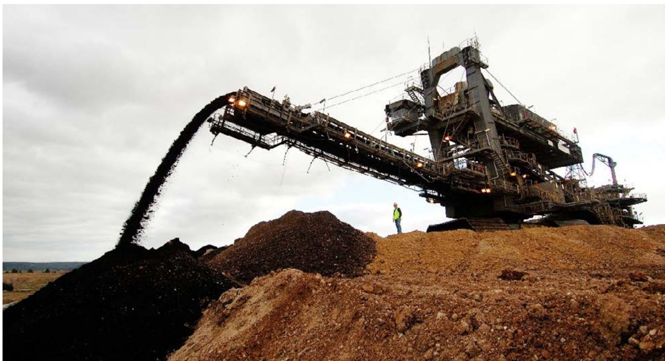
Image 2: Stacker distributing material on overburden site
