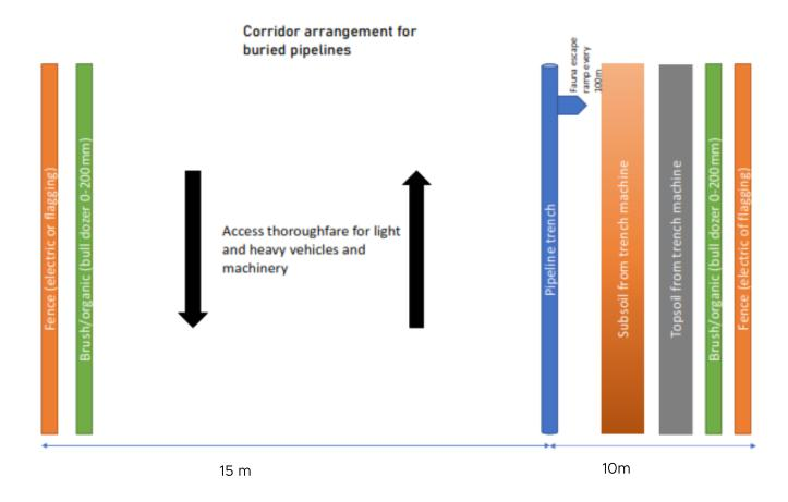
Figure 3: Schematic of Construction ROW (25m maximum width)
