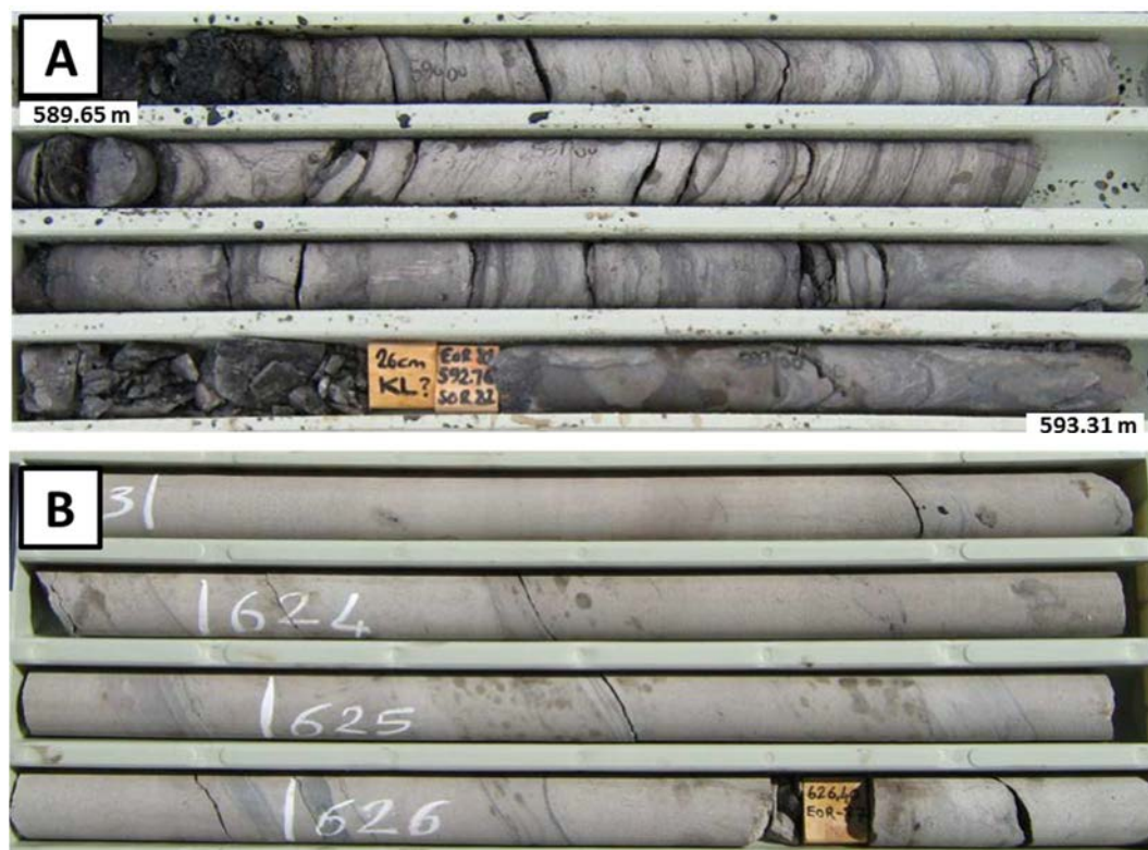
Figure 8.3 Photographs of drill core from Waukivory 1 showing (A) a high fracture density and slickensides associated within bedded siltstone and mudstone, and (B) relatively fractured sandstone. The width of the core trays is 1 m.
