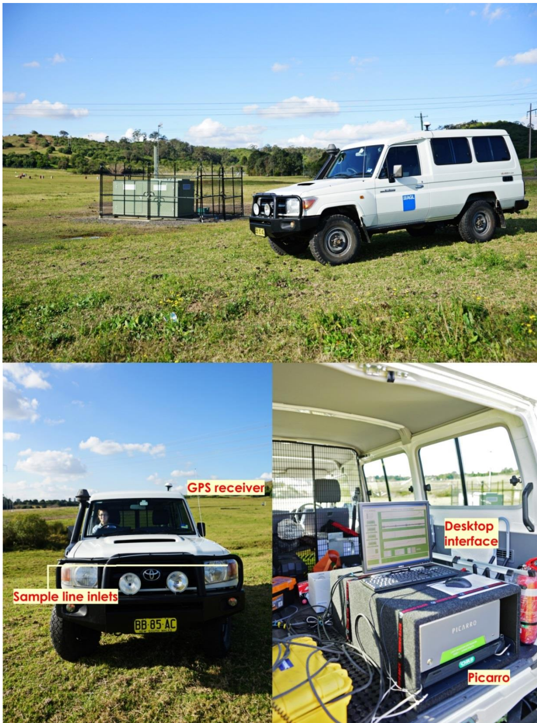
Figure 5-2: AGL mobile monitoring kit
