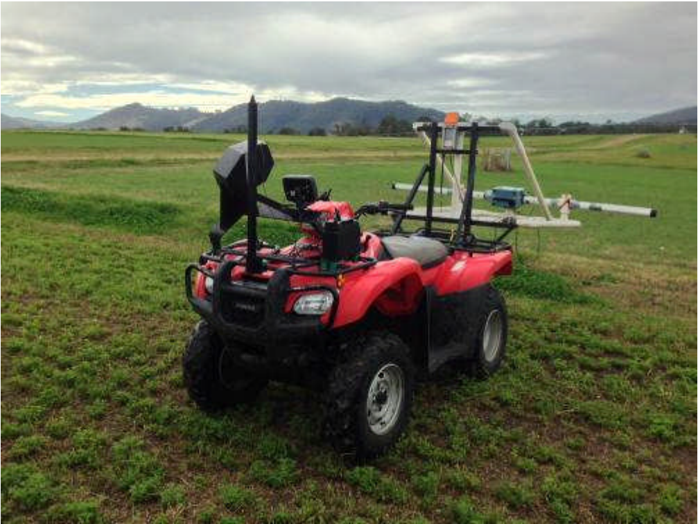
Plate 5: EM31 Unit Mounted to Quad Bike
