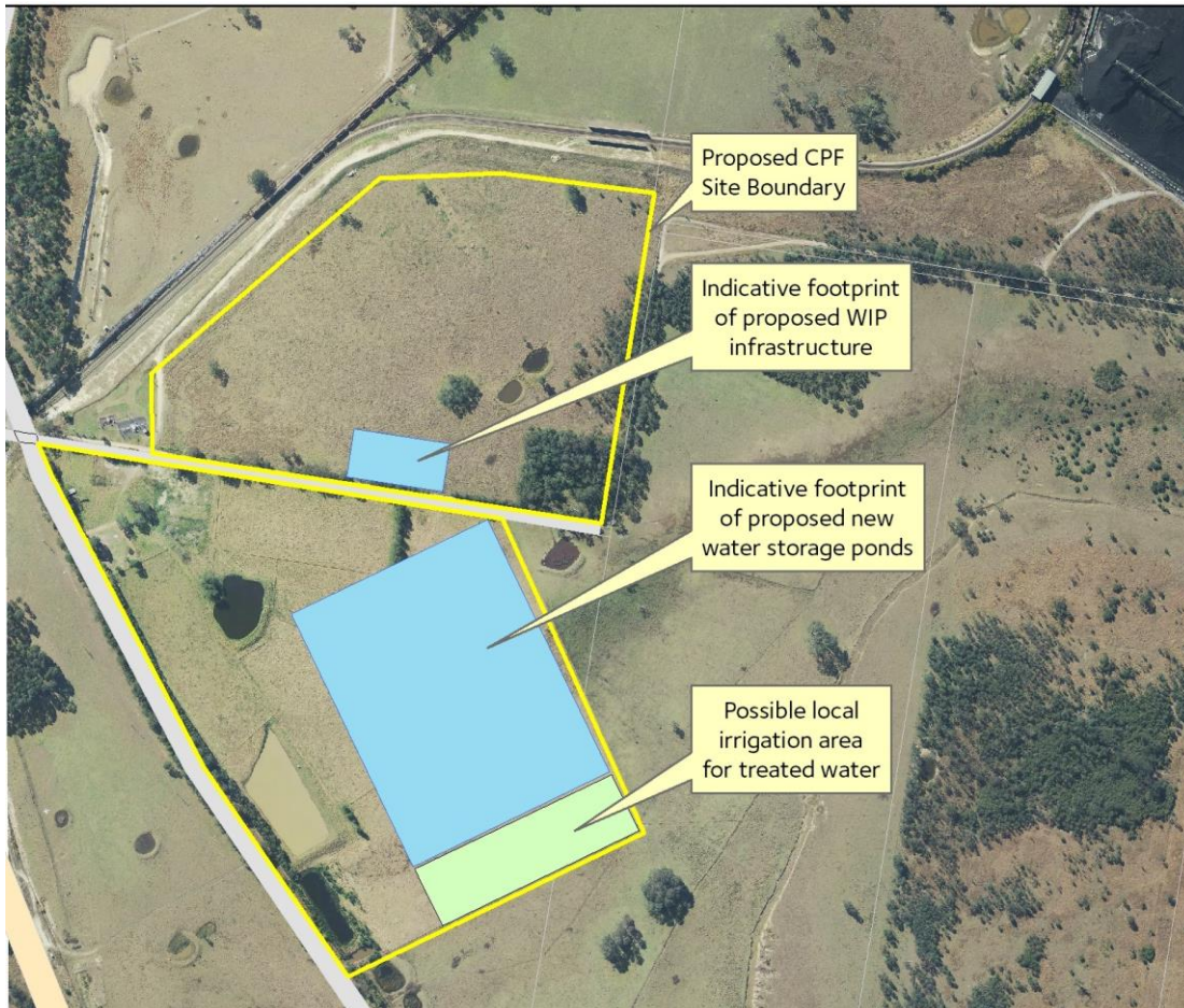
Figure 9.2: Indicative Layout of CPF Water Infrastructure (layout is subject to final design and approval)
