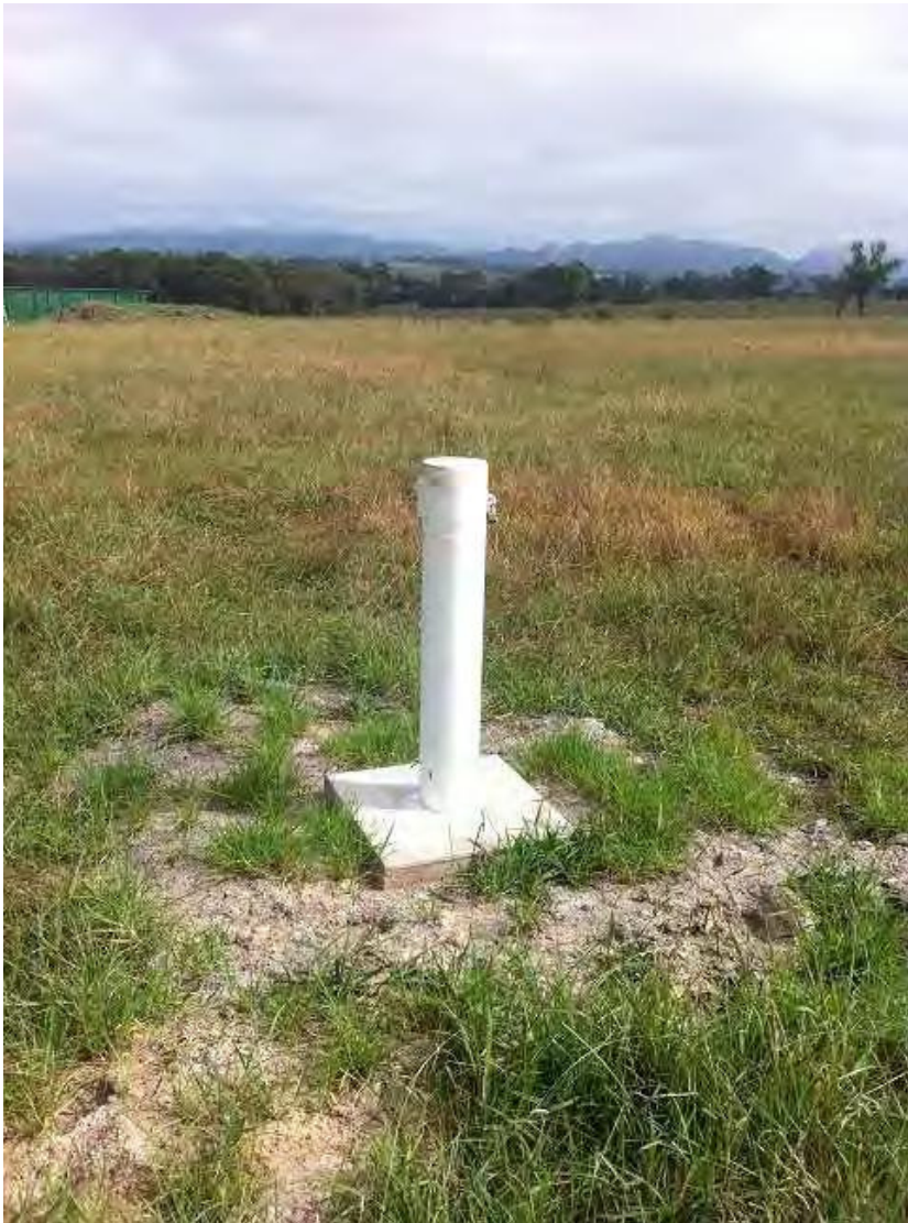
Plate 1 Example of an installed water monitoring bore
