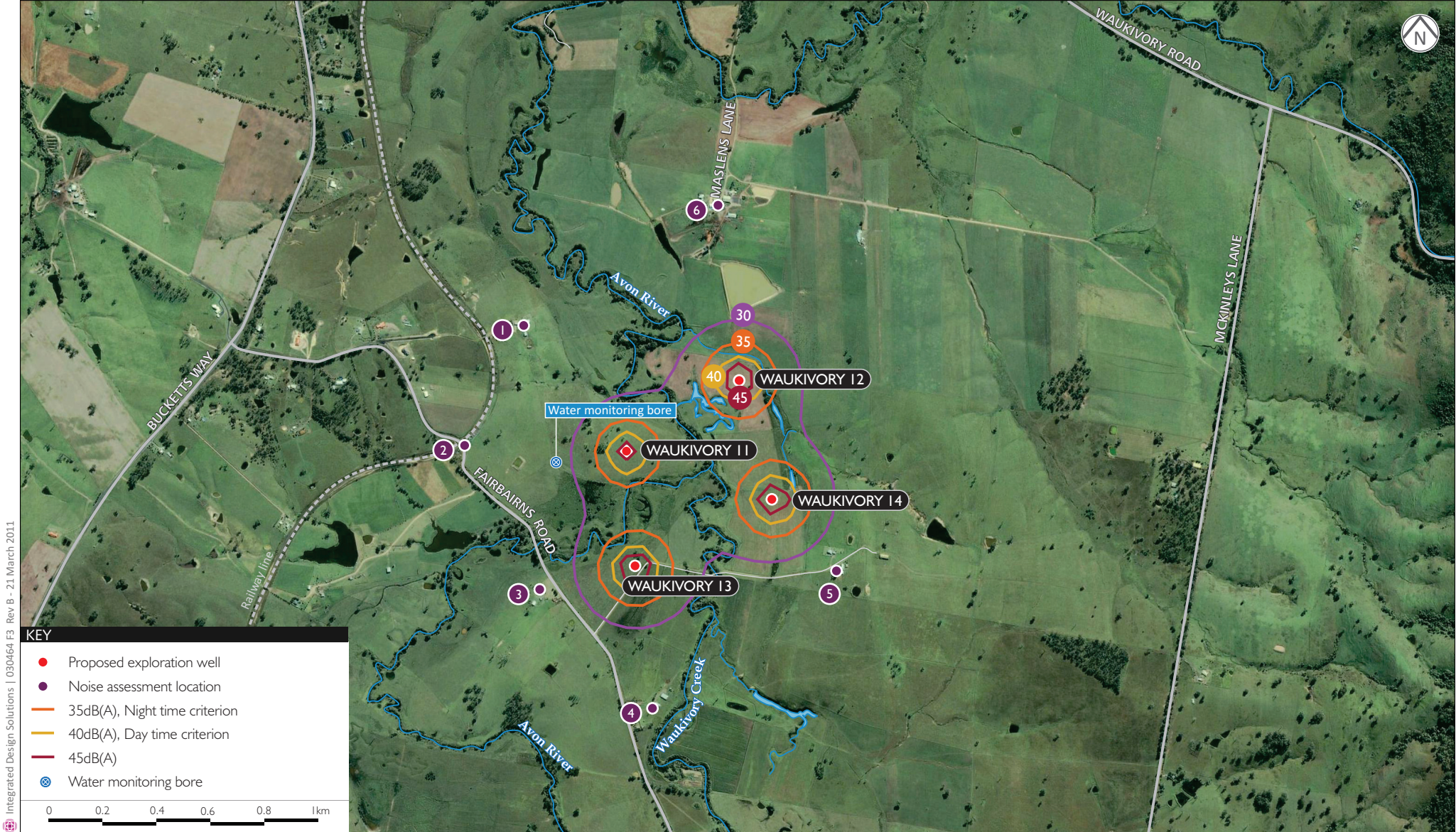
Predicted operational (Flaring) Leq noise levels from all wells combined, dB(A)
