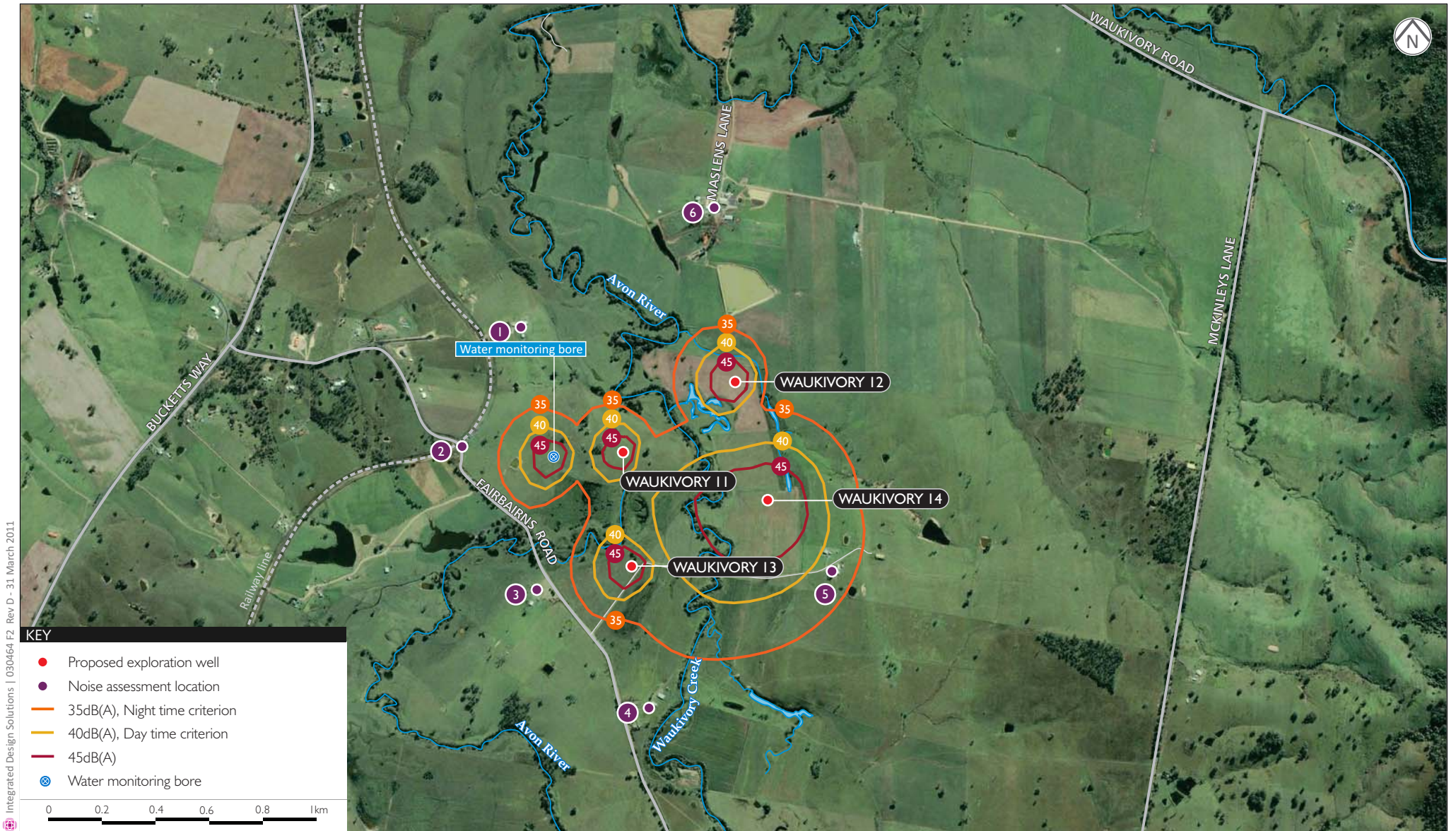
Predicted drilling outer envelope Leq noise levels - Mitigated drill and optimised layout dB(A)
