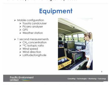
This slide shows my colleague Justine. I can show you the Picarro machine contained in the land cruiser car during the break. It also has a GPS to map where the methane measurements were taken. We also have a weather station so that if we are parked-up, we can put this out. If we get a peak, we can then determine what the wind speed and wind direction were at that location and from that back-calculate where that source may have been.
