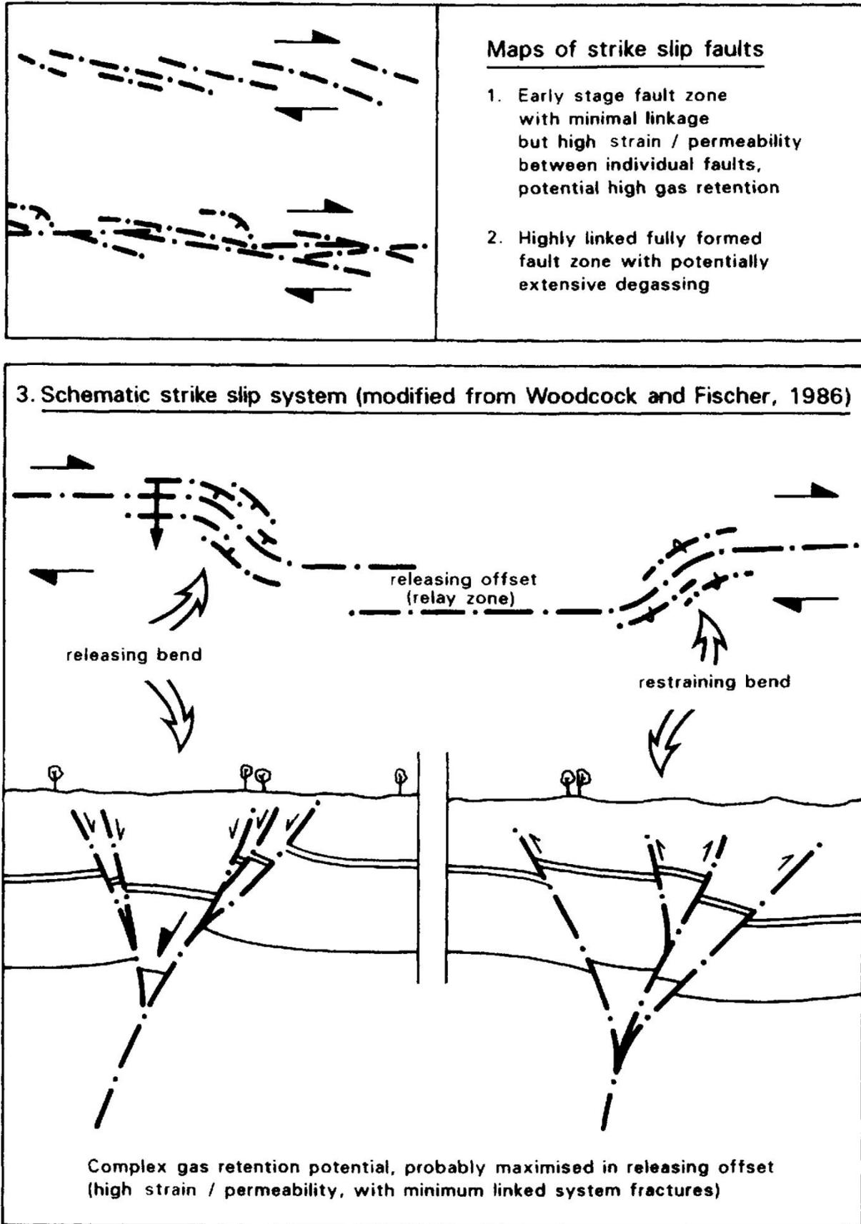
Figure 2.5 Strike slip fault examples illustrating the complex strain and permeability patterns (Woodcock & Fischer (1986) and Boardman and Rippon (1997)).
