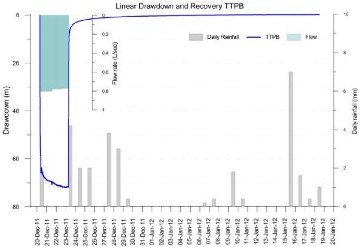
Figure 4.3 Linear plot of drawdown in TTPB versus time (minutes)
