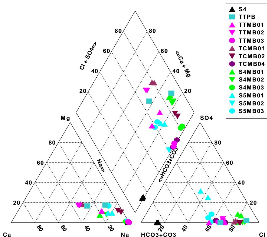
Figure 4.14 Piper diagram showing major ion chemistry for Stratford 4 gas well and monitoring bores
