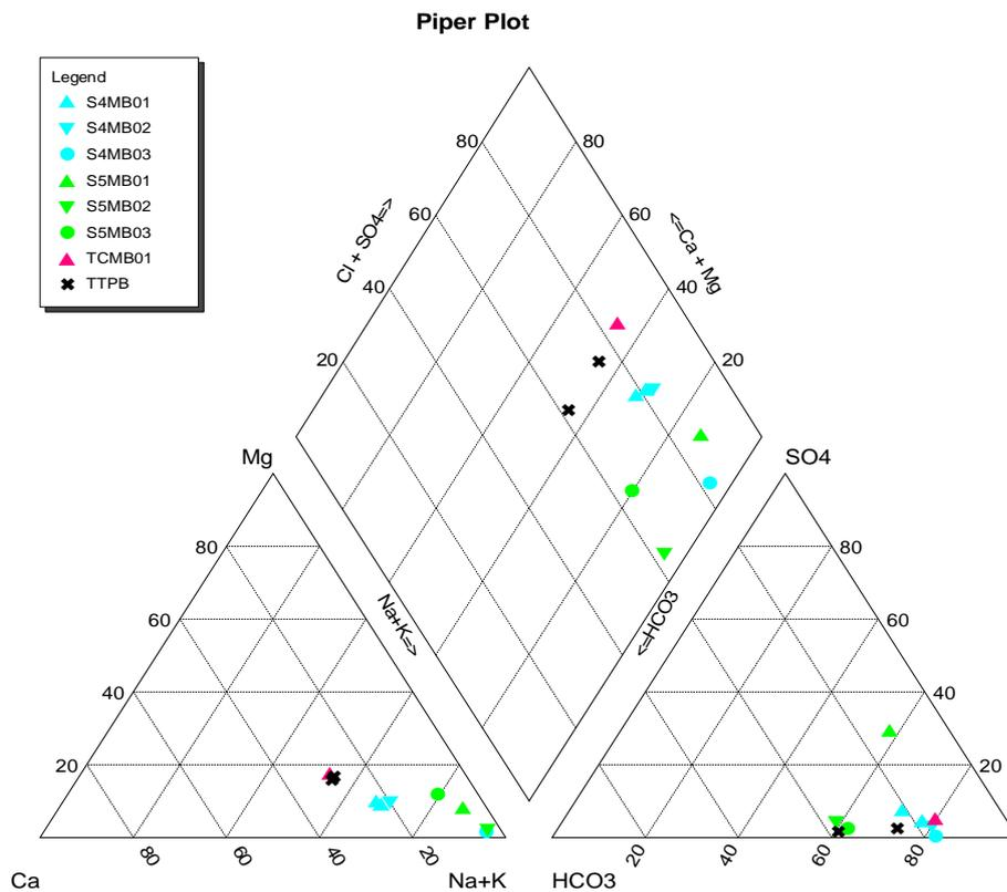
**Figure 4.10** Piper diagram showing major ion composition from TTPB (TTPB is compared to monitoring bores located outside the inferred fault zone)
