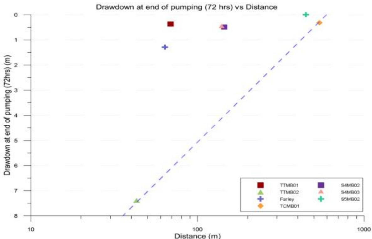
Figure 4.7 Plot of drawdown versus log distance from the pumping bore (TTPB). The dotted line represents the expected log-linear distance-drawdown relationship.
