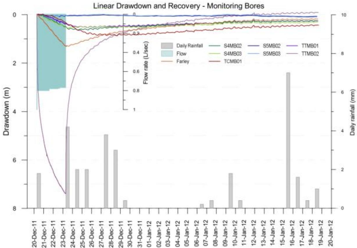
Figure 4.5 Linear plot of drawdown versus time at monitoring bores
