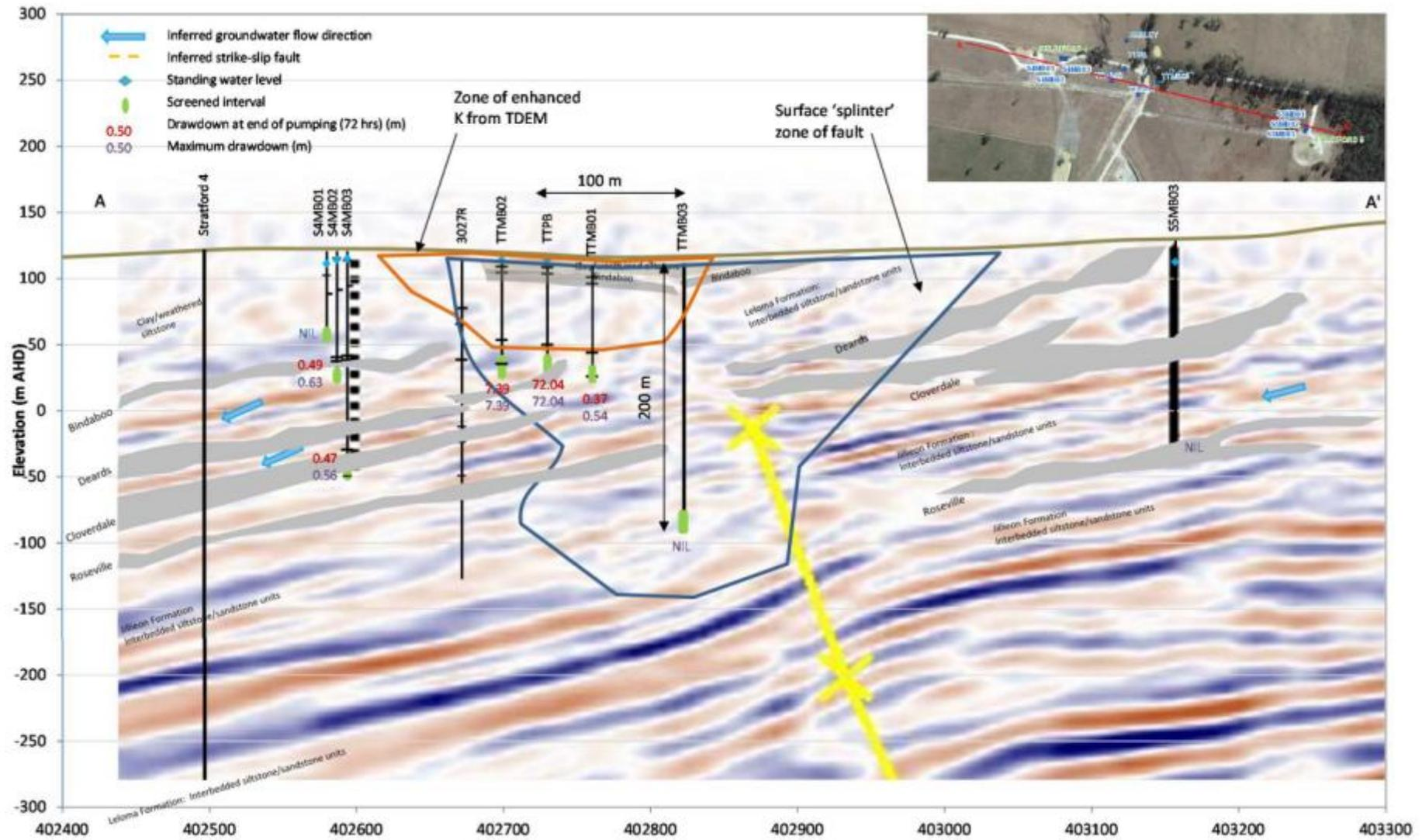
Figure 4.9 Cross-section showing the drawdown after 72 hours and maximum drawdown at each monitoring bore
