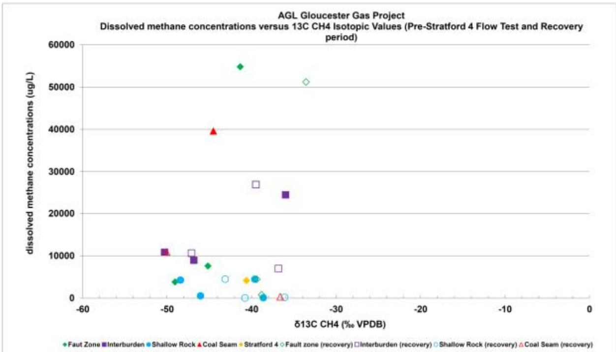
Figure 4.19 Plot of dissolved methane concentration versus carbon-13 ( $\delta^{13}\text{C-CH}_4$ ) in methane gas from monitoring wells and Stratford 4
