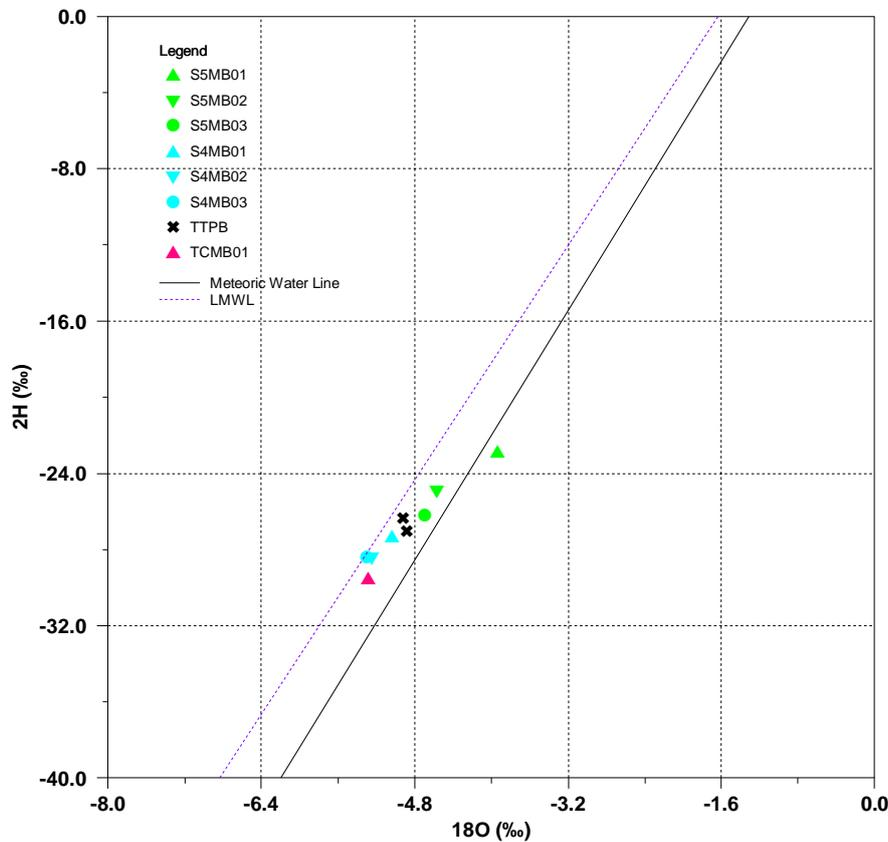
Figure 4.11 Bivariate plot of  $\delta 2H$  vs.  $\delta 18O$  showing stable isotope composition of TTPB, TCMB01 and nearby monitoring bores
