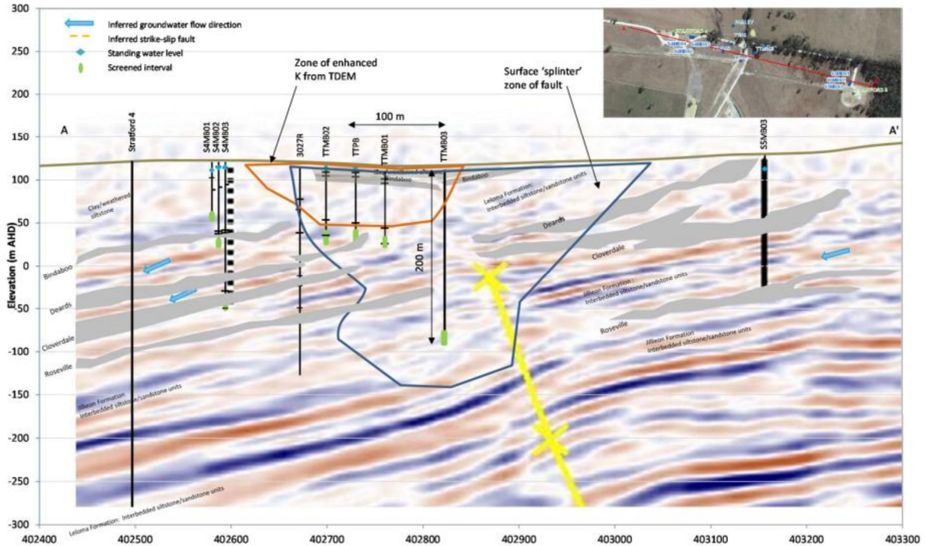
Figure 4.1 Cross-section (E-W), perpendicular to the fault zone, showing bore locations and geophysical interpretations
