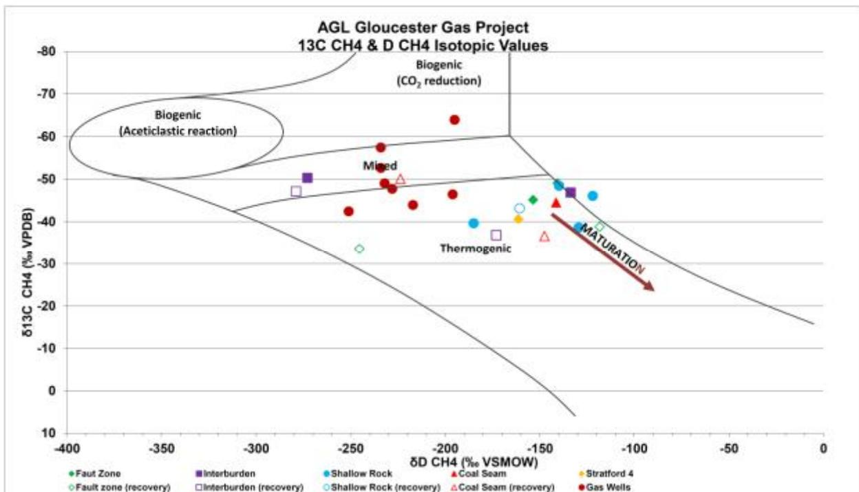
Figure 4.17 Plot of carbon-13 ( $\delta^{13}\text{C-CH}_4$ ) and deuterium ( $\delta^2\text{H-CH}_4$ ) in methane gas from monitoring wells and Stratford 4
