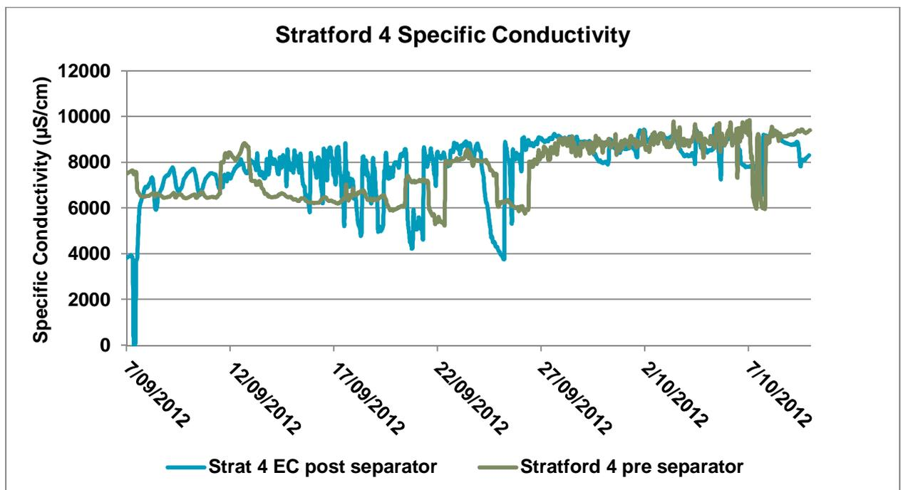
Figure 4.13 Stratford 4 specific conductivity during flow testing
