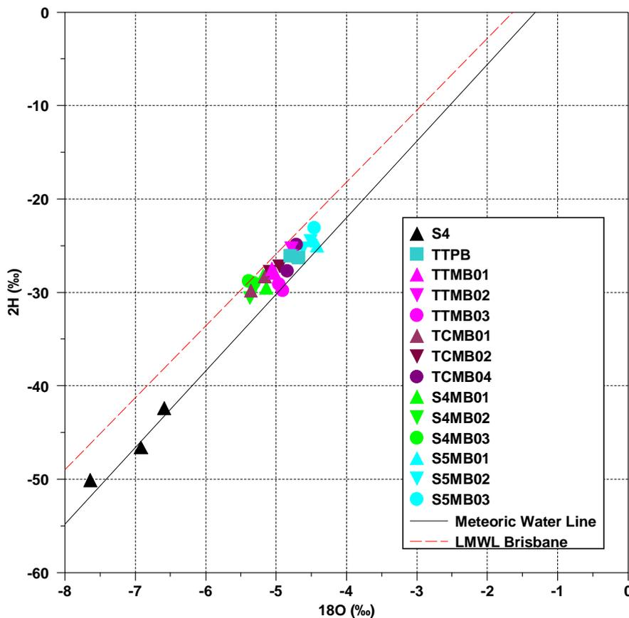
Figure 4.15 Bivariate plot of  $\delta 2H$  vs.  $\delta 18O$  showing stable isotope composition of Stratford 4 gas well and nearby monitoring bores
