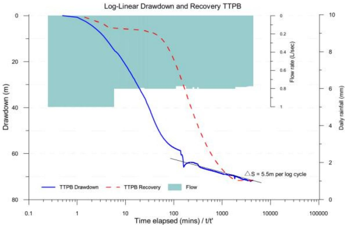
Figure 4.4 Log-linear plot of drawdown in TTPB versus time (minutes) and residual drawdown in TTPB versus  $t/t'$
