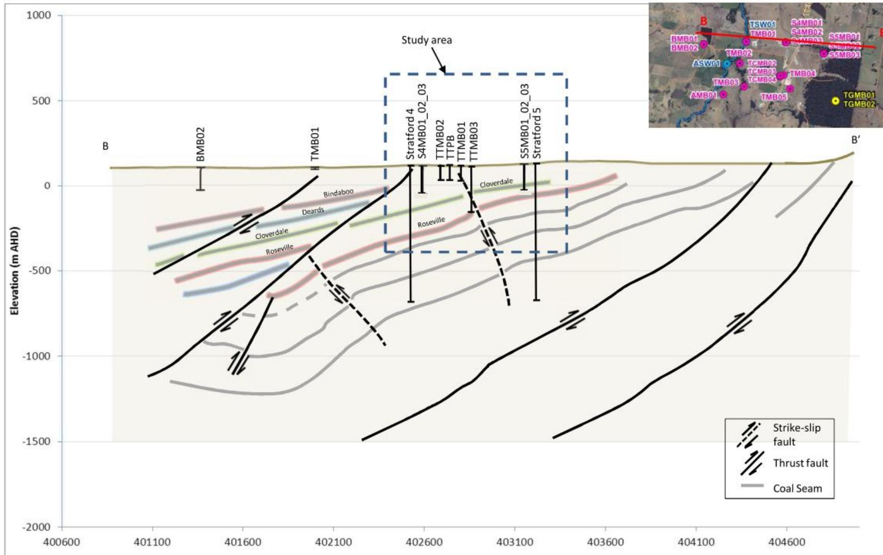
Figure 2.4 East-West schematic cross-section through the Stratford Pilot area
