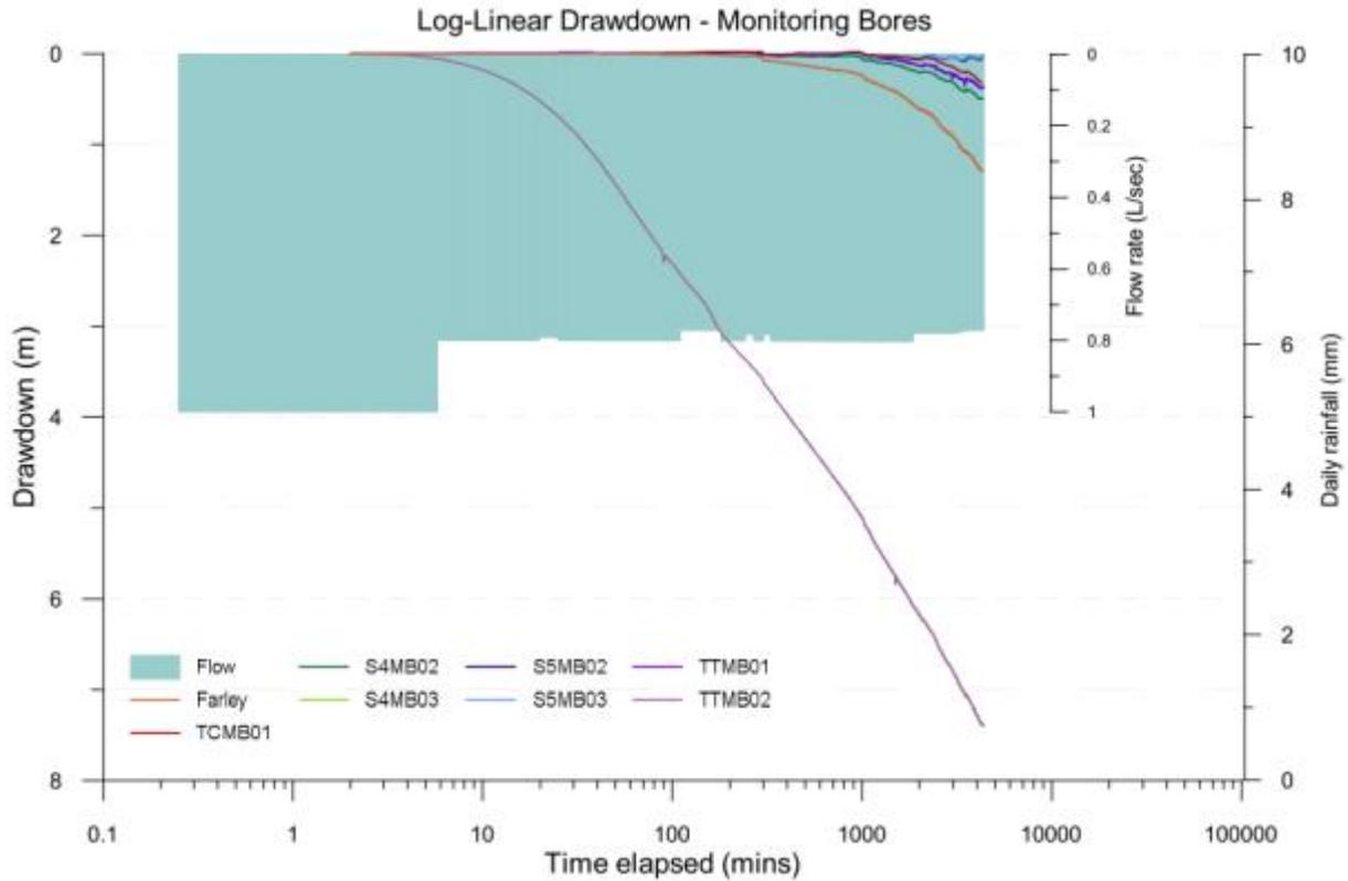
Figure 4.6 Log-linear plot of drawdown versus time at monitoring bores
