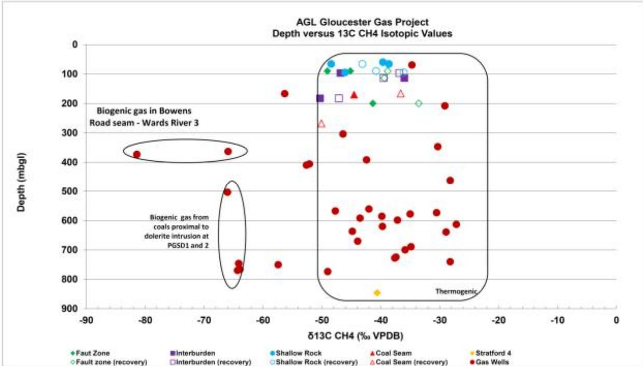
Figure 4.18 Plot of depth versus carbon-13 ( $\delta^{13}\text{C-CH}_4$ ) in methane gas from monitoring and gas wells
