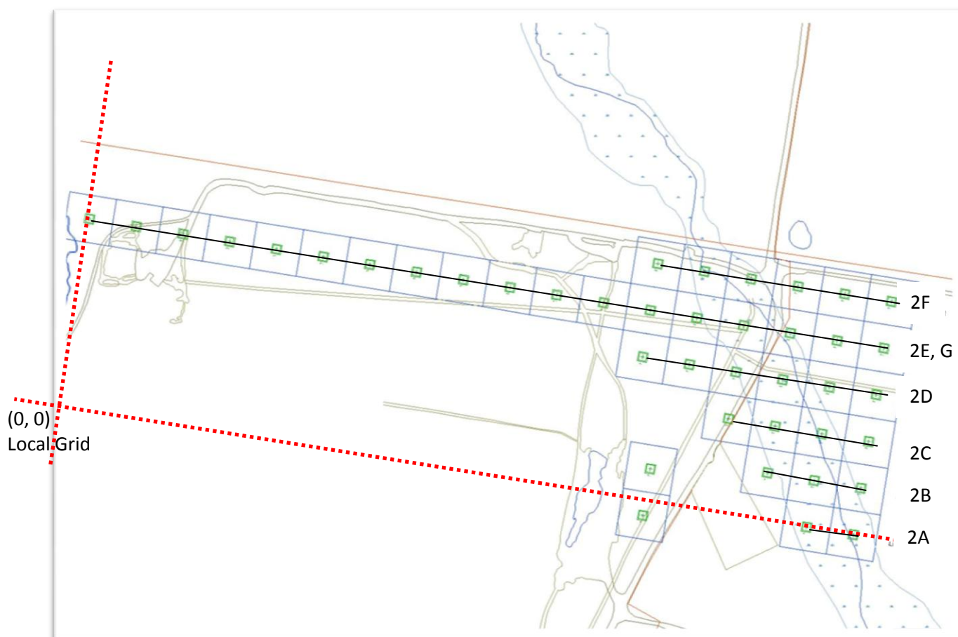
Image 2: Schematic of site. Showing origin and orientation of local grid (red dashed lines), Line Locations for pseudosections (black lines), Appendix reference numbers for pseudosections and location of transmitter loops (blue squares) and receiver locations (green points).
