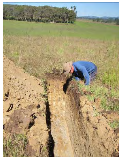
Plate 6. Inspecting soil profile in test pits
