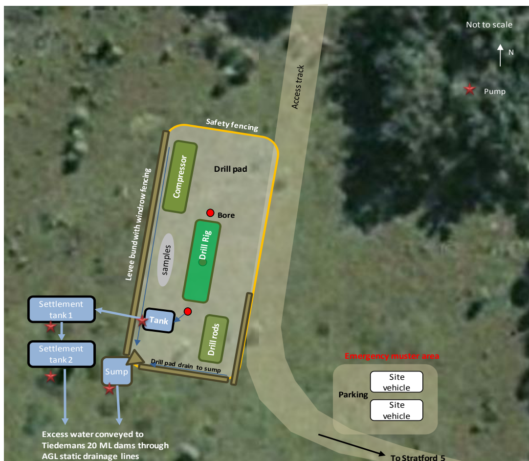
Figure 4-3 Typical drill pad layout
