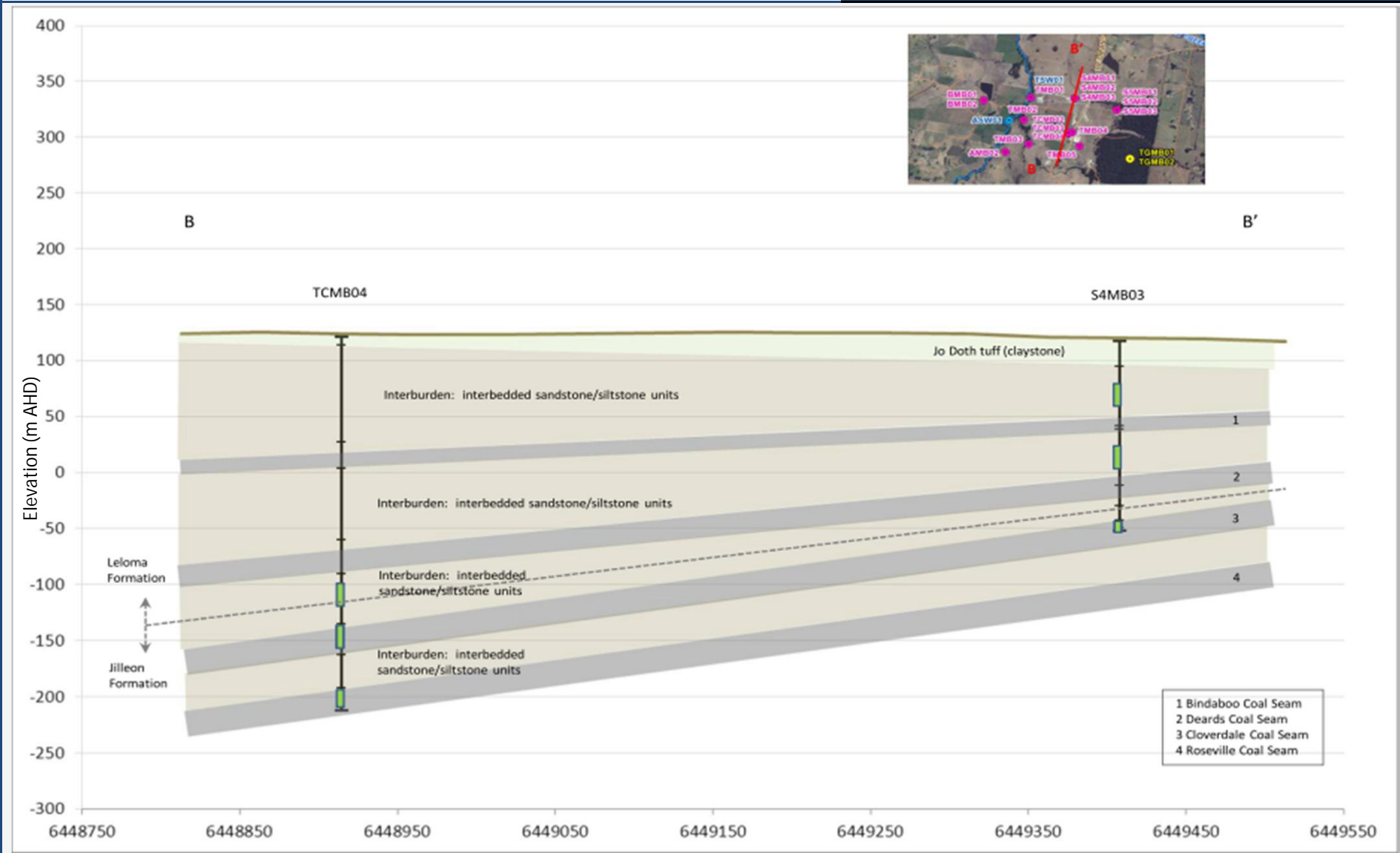
Figure 5-4 Geological cross-section through the Tiedman property (N-S)
