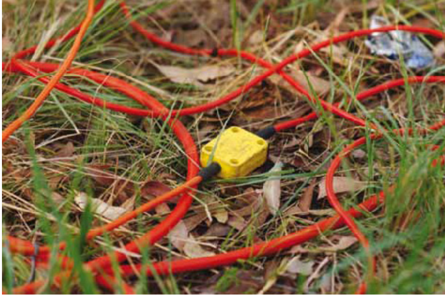
Figure 2.4 Geophone and cabling (Source: AGL Fact Sheet, 2011)
