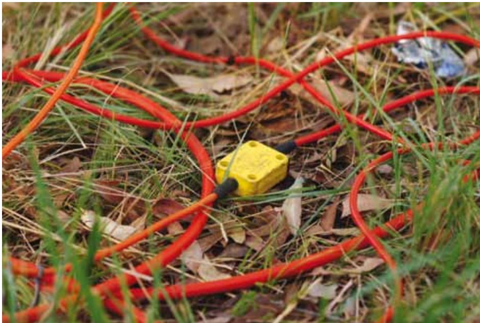
^ A geophone in the ground.
