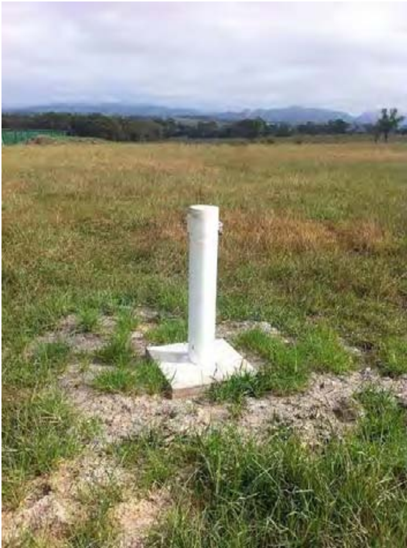
Plate 1 Example of an installed water monitoring bore
