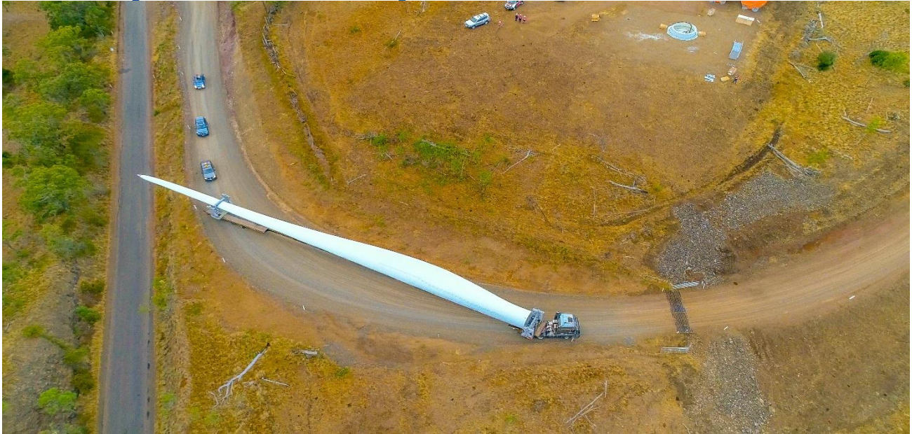
Transportation of blade on site
