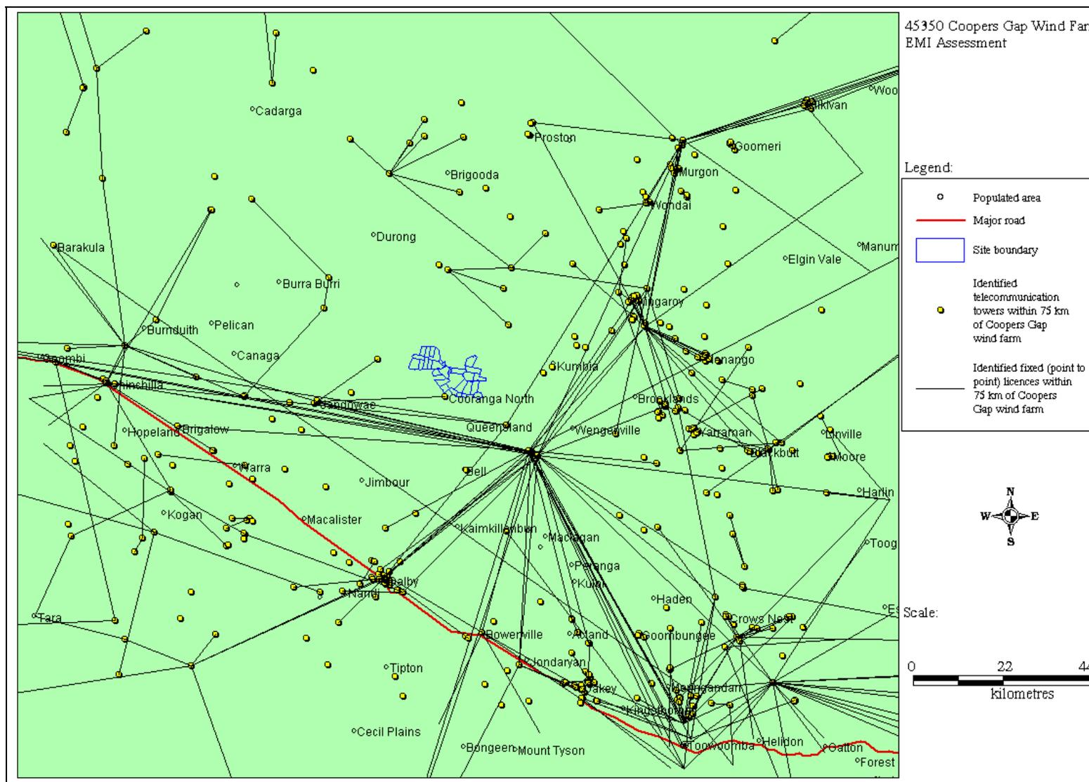
Figure 4 Identified transmission vectors for fixed licences of point-to-point type proximate to Coopers Gap wind farm
