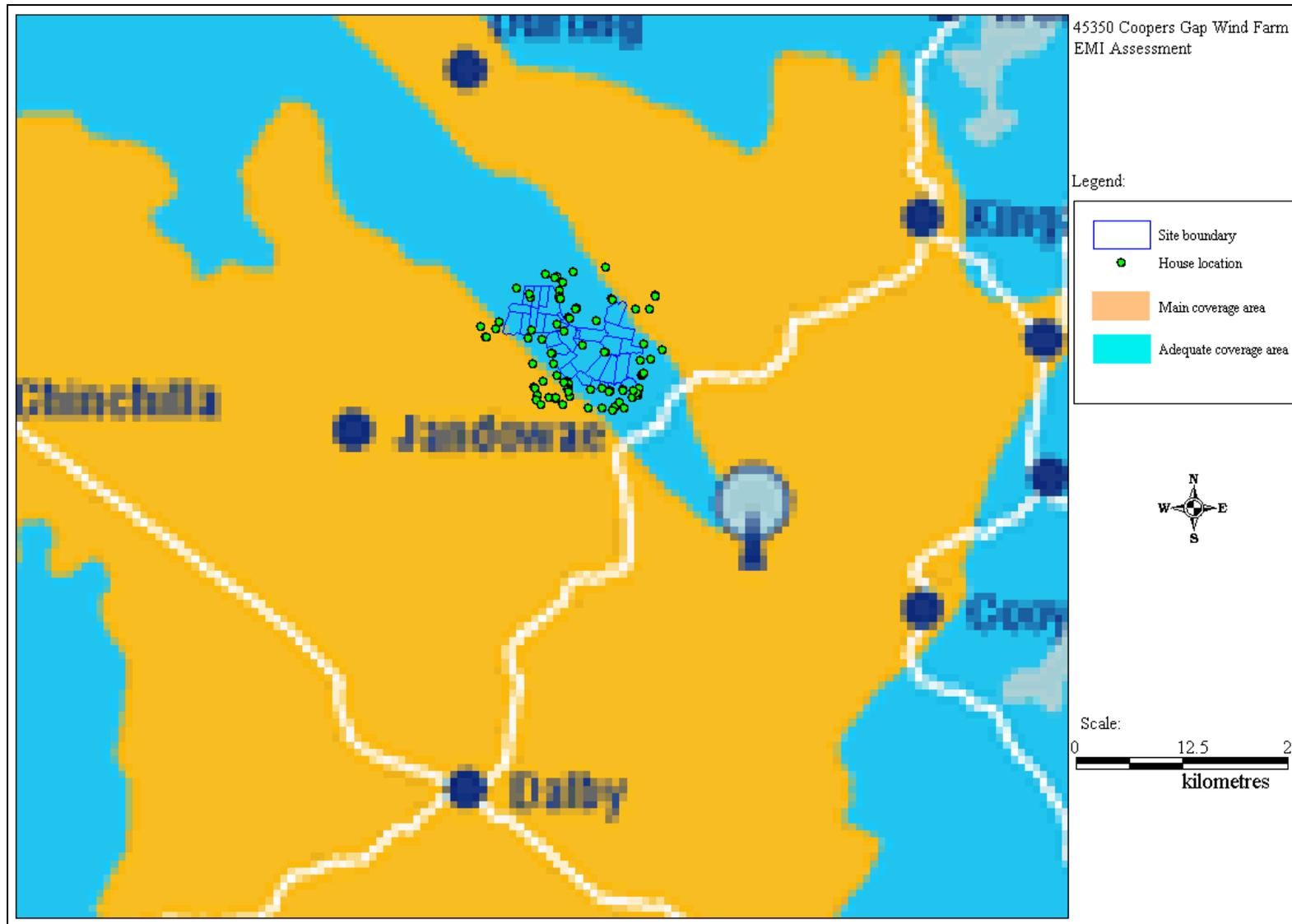
Figure 12 Digital TV coverage from Darling Downs transmitter at Mt Mowbull
