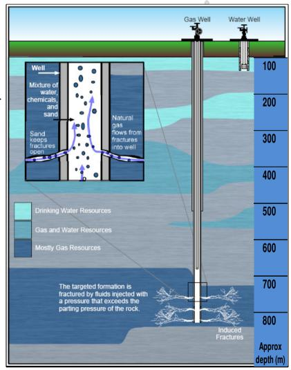
Figure 2 Stratigraphy of Southern Sydney Basin (from Geological Survey of NSW, 1996) and Generalised Illustration of CSG well (modified from USEPA 2011)
